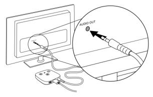
If your TV loudspeakers switch off when connected with the analog 3.5mm audio cable, use the optical audio cable instead (see: "Connecting with optical cable").
