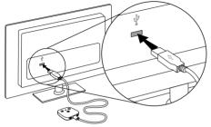
The TV Connector will turn ON the first time it is connected to a power source. If the TV Connector does not turn ON automatically when the power supply is connected, press and hold the power button for 2 seconds to turn ON the device.
